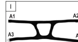
Place headgear with Velcro side down on a flat surface. Detach 2 Velcro tabs on A1 & A2.
